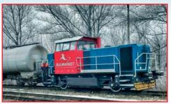
MDD 4-00 locomotives are the workhorse for any in-yard industrial shunting works and could also be used for hauling light trains on main line. MDD 4-00 has very high start tractive effort and keeps the optimum power to weight ratio.
