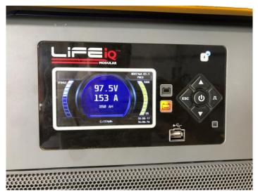
The powerful Life-iQ battery charger is securely integrated on board. It allows full battery recharge in just 5,5 hours.
